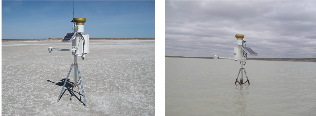
Figure 2. Sampling system resting on a dry and a wet playa at Yellow Lake.
